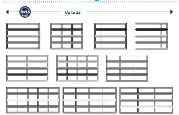
The placement of vertical mullions and the height of the glass sections can be adjusted to suit the desired architectural look.
